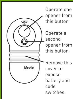
To operate your opener from the smaller button, match the code switches, but reverse code switch #1 in the remote control. To operate an opener from each button, set the same code in each opener, but then reverse code switch #1 in one opener.
